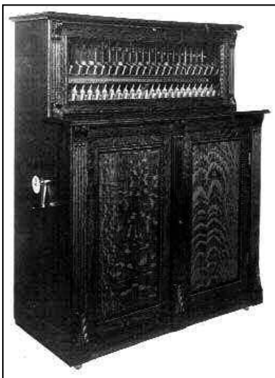
Figure 4. A companion to the deKleist tubular piano was this one featuring piano-type hammers sounding a set of flat metal bell bars.
